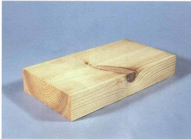
Figur 6: Hornkvist Figure 6: Splay knot
