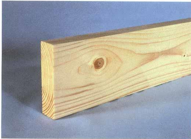
Figur 11: Gjennomgående flatsidekvist Figure 11: Through face knot
